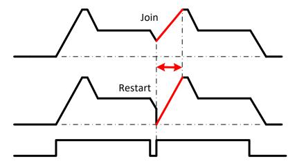
The J/R setting has no effect on the attack duration; only the attack slope will vary as needed.
