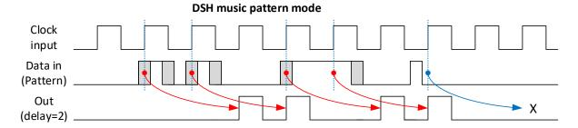
By maintaining the Xtra button pressed, you can set by how many steps the pattern will be delayed. Turning the pot within its first half, the LED column indicates the delay as follows:
