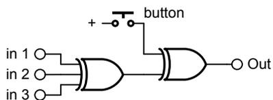
Xor can be used as a “digital ring modulator” such as implemented in the ARP Odyssey and KORG MS-20 synthesizers. Feed two inputs with two oscillators to get the effect.
